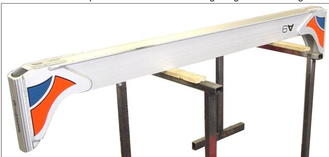
2. Take the measure of the the widthnes on the outside of the chassieframe and add 6 mm. Example: If the frame withnes is 1250 mm, must the space between the attachment framestop be 1256 mm.
