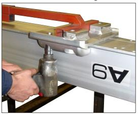
NOTICE! It's wery important to retighten the screwer a short time after that the equipment has started to be used.
