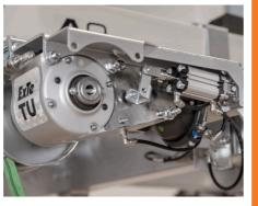
The air-operated release mechanism is mounted directly adjacent to the tensioner. When the stack is about to be bound, the tensioner is released so that the sling can be lifted using a crane or grab. Uncoupling can be effected via either an operation from the cab or by using the remote control. Quickly, smoothly and safely.
