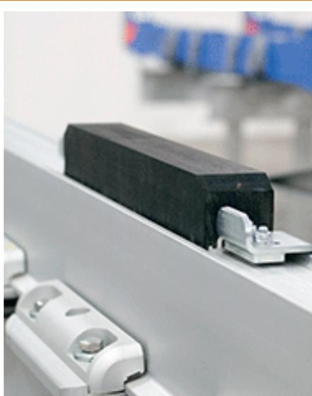
When idling, the crane rests on a bunk. Bunks and crane booms get damaged and worn during transportation. The design of the crane guard, with a robust rubber girder attached to the bunk, absorbs shocks and vibrations, thereby protecting against damage.
