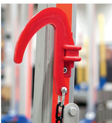
The hook has been designed so it can be easily lifted with the grapple. Both the hook and the holder are made from specially-designed, durable rubber. The holder is easy to mount on the stake and has been designed to ensure the hook remains in place even during transportation. Our hook solution is gentle on the body and increases safety, while also speeding up the lashing process.
