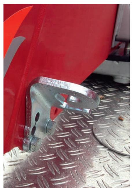
Both the hooks and hoops are made from high-tensile steel. They are bolted to the release mounting.
