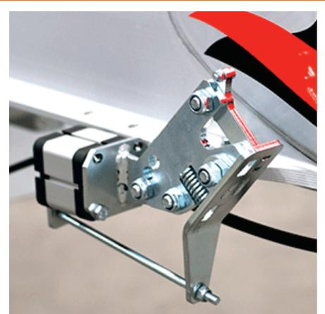
The benefit of a pneumatic release mechanism is that the driver does not have to walk round and release every single lashing individually. Using just one hand, from inside the cab, the lashings on all of the stacks can be released simultaneously. Once the lashings have been released, the strap coils up automatically. Simple and practical. If you only need to release the lashing on individual stacks, then you still have the cable release.
