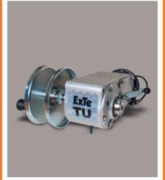
On timber rigs, TU tensioners are mounted onto bunks or chassis frames. The symmetric design (right/left) means that drums, as well as release levers, can be attached to either side, depending on specific needs or preferences. The TU tensioner has been designed to secure all types of heavy cargo for transportation, whether it be timber or any other type of cargo.
