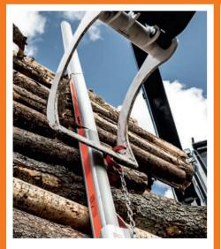
The hook has been designed so it can be easily lifted with the grapple. Both the hook and the holder are made from specially-designed, durable rubber. The holder is easy to mount on the stanchion and has been designed to ensure the hook remains in place even during transportation. Our hook solution is gentle on the body and increases safety, while also speeding up the lashing process
