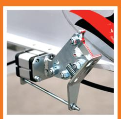
The benefit of a pneumatic release mechanism is that the driver does not have to walk round and release every single lashing individually. Using just one hand, from inside the cab, the lashings on all of the stacks can be released simultaneously. Once the lashings have been released, the strap coils up automatically. Simple and practical. If you only need to release the lashing on individual stacks, then you still have the cable release.
