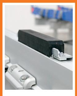
When idling, the crane rests on a bunk. Bunks and crane booms get damaged and worn during transportation. The design of the crane guard, with a robust rubber girder attached to the bunk, absorbs shocks and vibrations, thereby protecting against damage.
