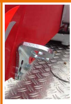
Both the hooks and hoops are made from high-tensile steel. They are bolted to the release mounting.
