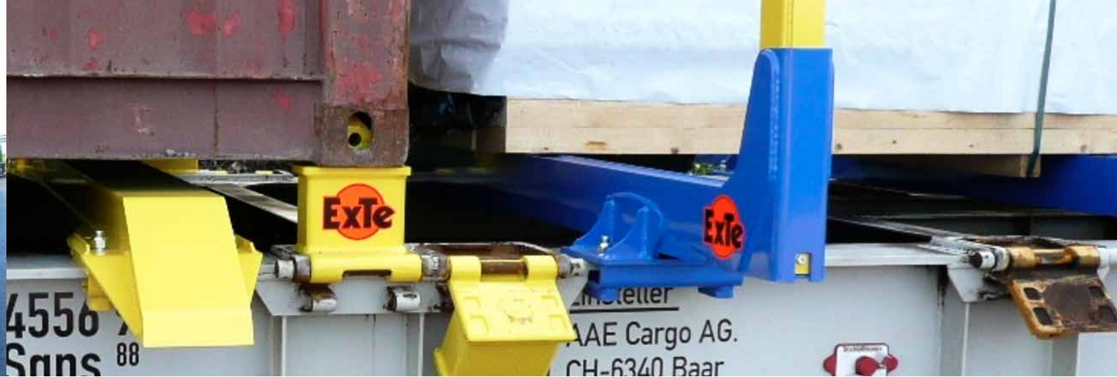
The ExTended container spigots (the equipment pictured above) lift containers above timber bunk bolsters and support bolsters.
